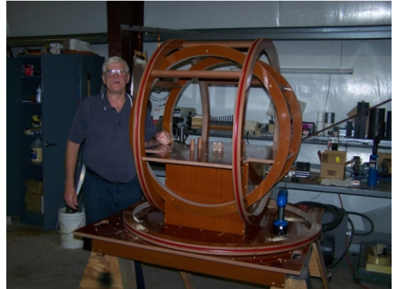
Tri-axial Helmholtz coil.
