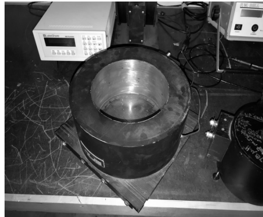
Super coil fixture to magnetize ring magnets for audio speakers.
